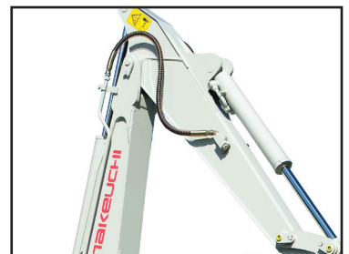
Auxiliary Hydraulic Lines
